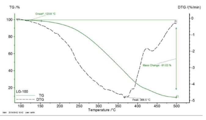
The heating and degradation of LG100 demonstrates that the product has a non-linear exothermic pyrolysis process, meaning that as the equipment to which the grease is applied is partially insulated from heating while the equipment is operating. In effect, the grease withstands incremental increases in temperature without degrading or oxidising and continues to protect the equipment throughout high temperature processing.
